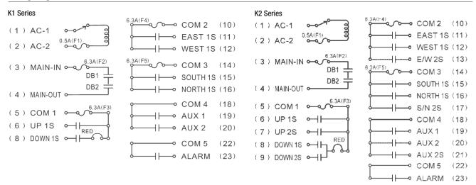
Please Note: Shown are the "default" wiring diagrams. If custom programming has been done, this might alter the relay outputs. See Manual for DC wiring diagrams.
